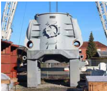
Service coal mill
